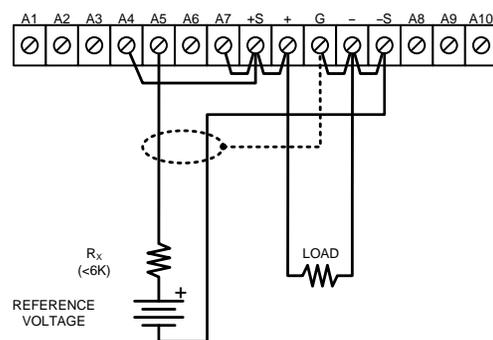
Figure 3-4. Remote Voltage Programming (Constant Voltage)
