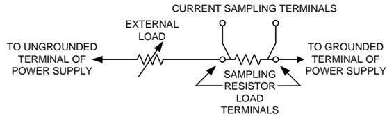
Figure 5-2. Output Current Measurement Technique
