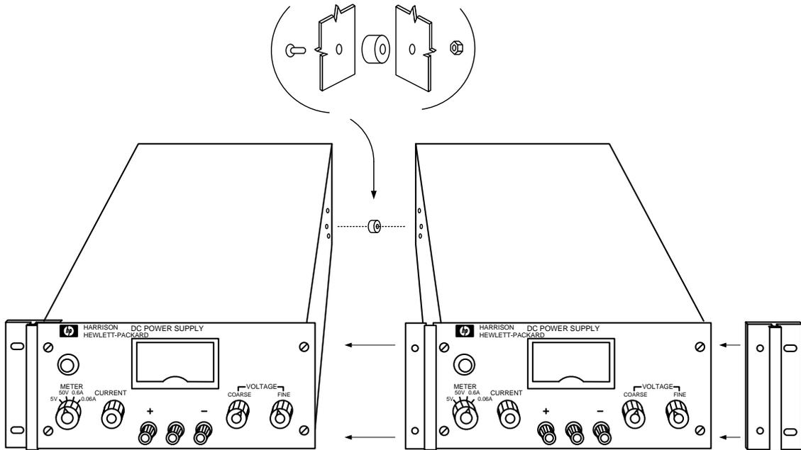
Figure 2-2. Rack Mounting, Two Units
