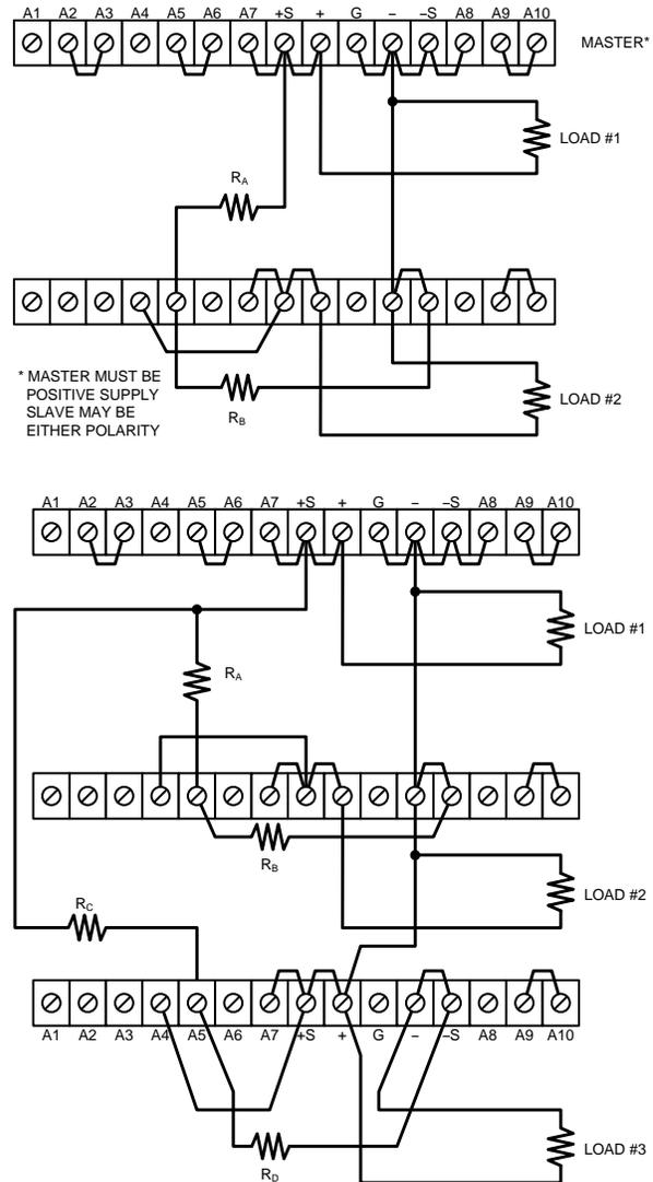
Figure 3-10. Auto-Tracking. Two and Three Units
