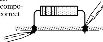
In the event that either the circuit board has been damaged or the conventional method is impractical, use method shown below. This is especially applicable for circuit boards without eyelets.
