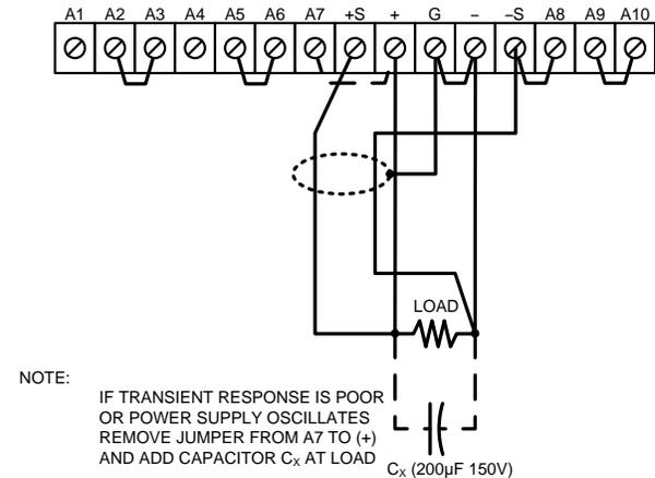
Figure 3-6. Remote Sensing
