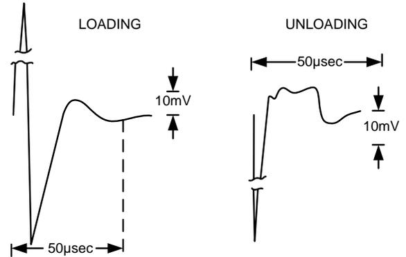
Figure 5-8. Transient Recovery Time, Waveforms
