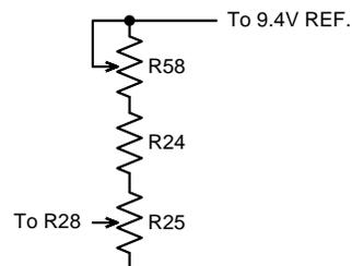
The above changes have been made to allow for Option 040 (multiprogrammer remote programming) operation; to allow the current limit to be set to 110  $\pm$ 2% of rated current.
