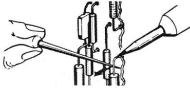
2. Reheat solder in vacant eyelet and quickly insert a small awl to clean inside of hole. If hole does not have an eyelet, insert awl or a #57 drill from conductor side of board.
