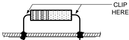
2. Bend protruding leads upward. Bend lead of new
