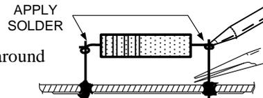
This procedure is used in the field only as an alternate means of repair. It is not used within the factory.
