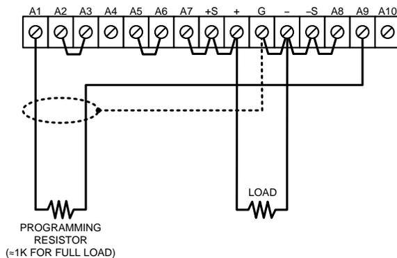
Figure 3-5. Remote Resistance Programming (Current Limit)
