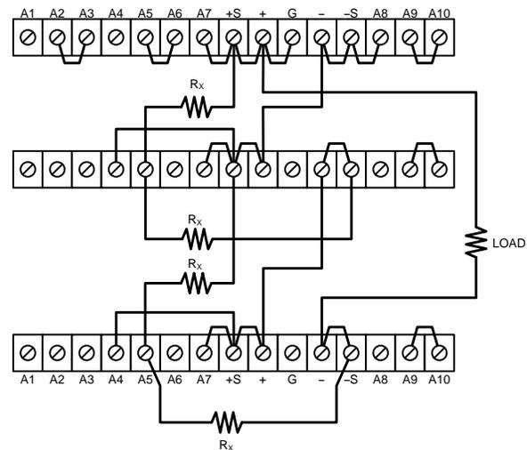
Figure 3-8. Auto-Series, Two and Three Units
