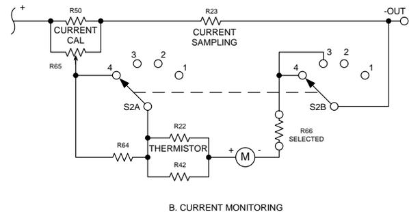
Figure 4-3. Meter Circuit, Simplified Schematic
